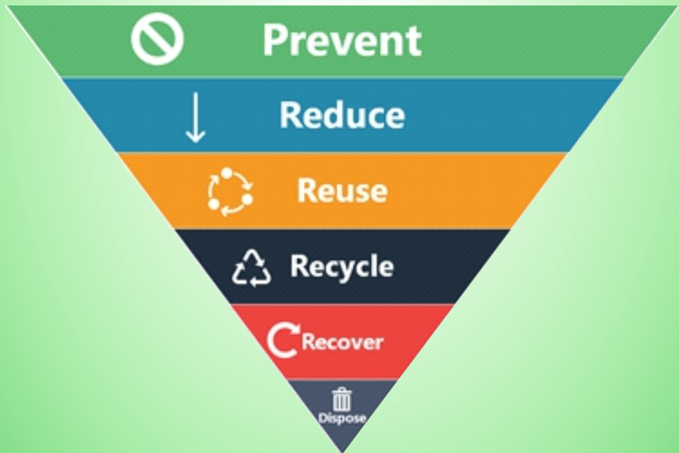
Fig.1.Waste Hierarchy Pyramid (from the most favourable (top) to the least (bottom) Waste minimization at source (prevention)
