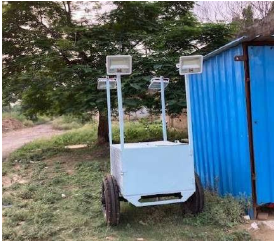
Trolley mounted emergency lights
