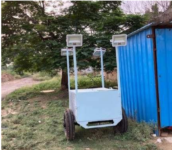
Trolley mounted emergency lights
