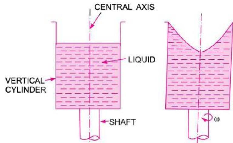
(a) CYLINDER IS STATIONARY (b) CYLINDER IS ROTATING
