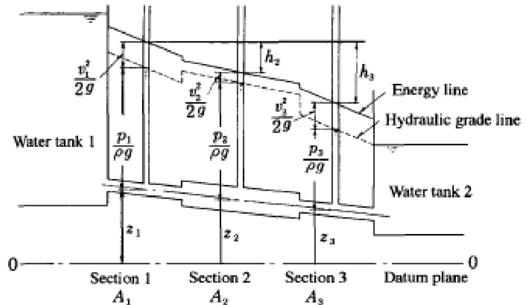
Fig. 5.7 Hydraulic grade line and energy line
