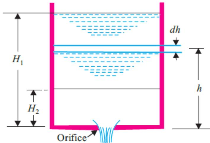
Fig. 8.13 Tank with an orifice at its bottom.
