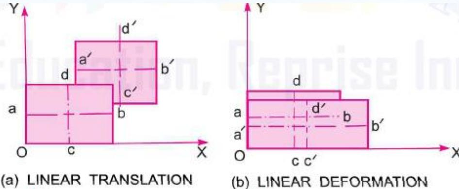
**5.9.1 Linear Translation.** It is defined as the movement of a fluid element in such a way that it moves bodily from one position to another position and the two axes  $ab$  and  $cd$  represented in new positions by  $a'b'$  and  $c'd'$  are parallel as shown in Fig. 5.11 (a).
