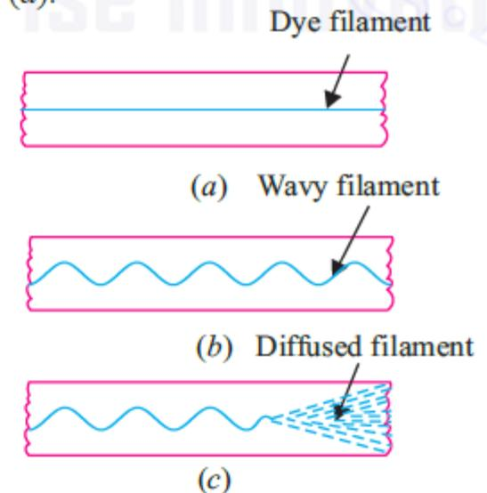
**Fig. 10.2.** Appearance of dye filament in (a) laminar flow, (b) transition, and (c) turbulent flow.
