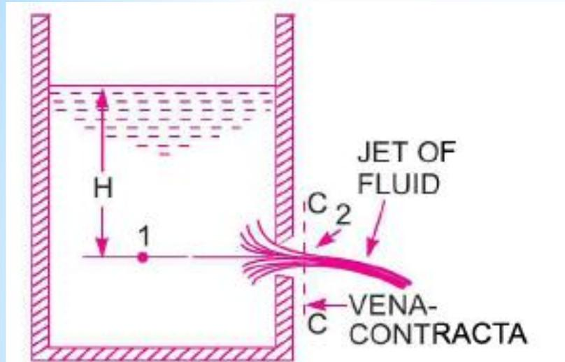
fig. 7.1 Tank with an orifice.
