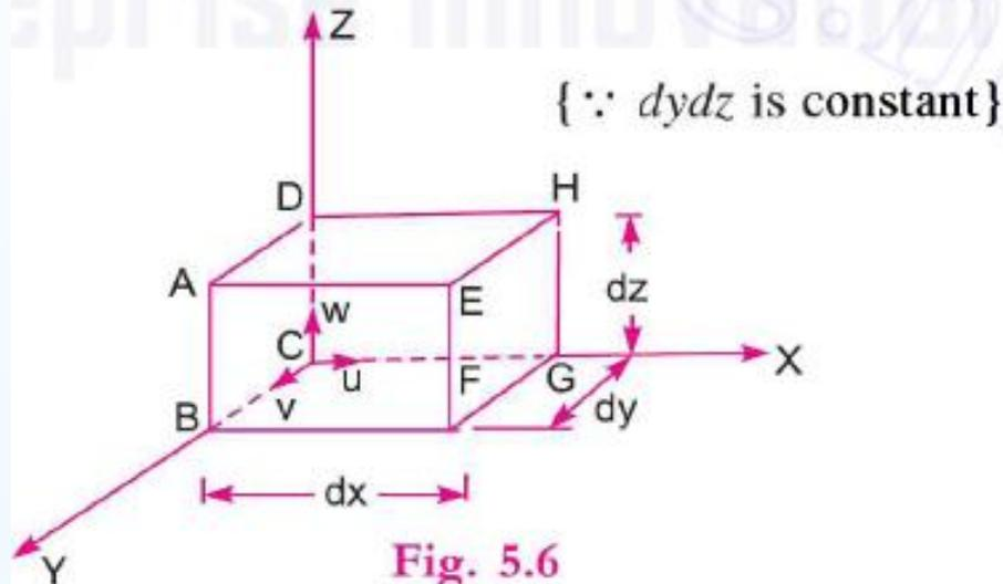
Consider a fluid element of lengths  $dx$ ,  $dy$  and  $dz$  in the direction of  $x$ ,  $y$  and  $z$ . Let  $u$ ,  $v$  and  $w$  are the inlet velocity components in  $x$ ,  $y$  and  $z$  directions respectively. Mass of fluid entering the face  $ABCD$  per second
