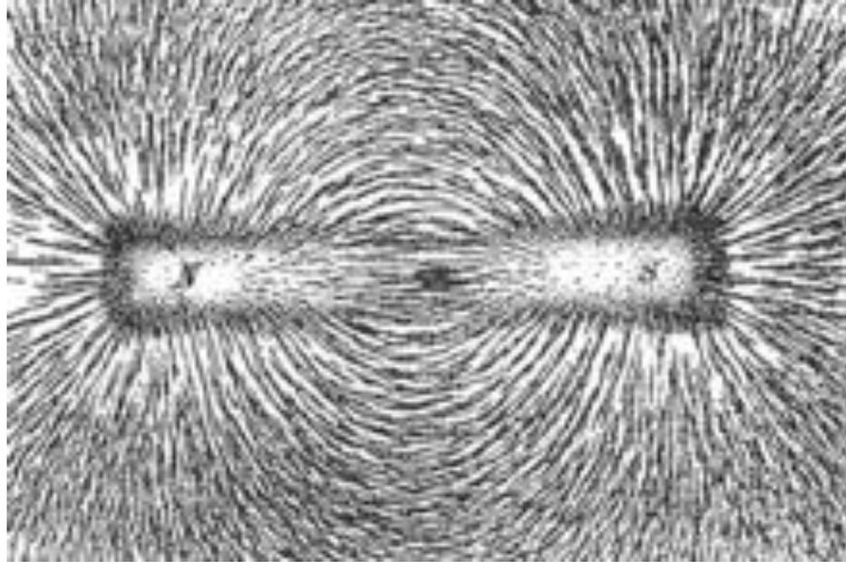
The direction of [magnetic field](#) lines are streamlines represented by the alignment of [iron filings](#) sprinkled on paper placed above a bar magnet
