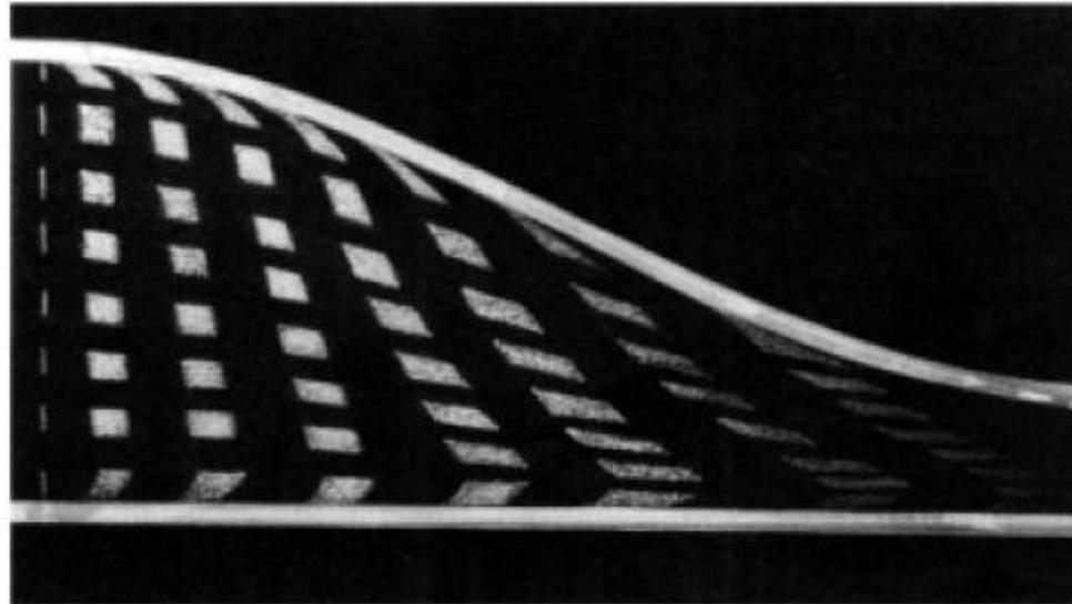
Deformation and rotation of fluid particles running through a narrowing channel
