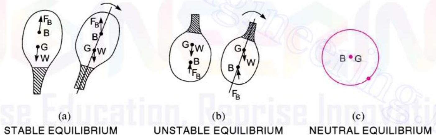
Fig. 4.12 Stabilities of sub-merged bodies.
