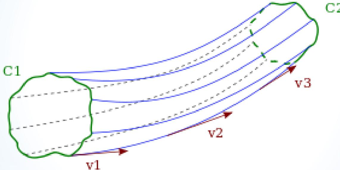
Solid blue lines and broken grey lines represent the streamlines. The red arrows show the direction and magnitude of the flow velocity. These arrows are tangential to the streamline. The group of streamlines enclose the green curves to form a stream surface.
