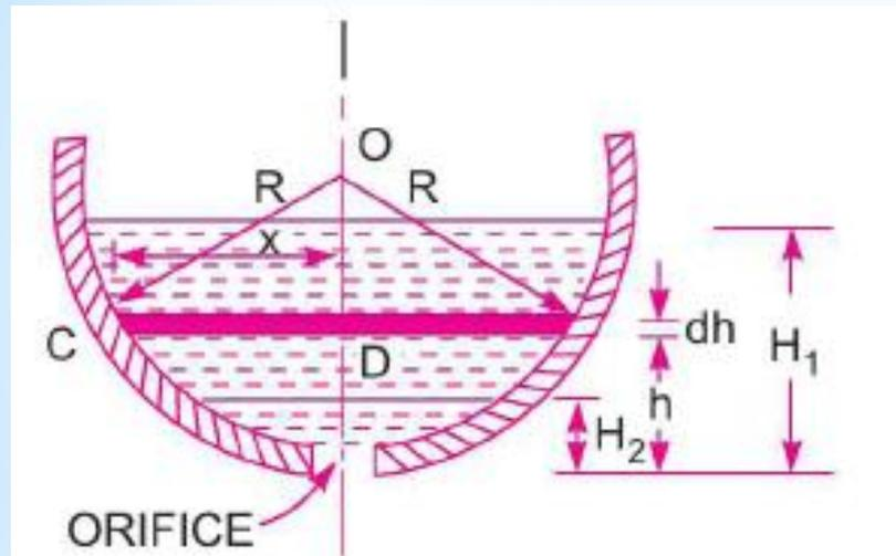
$$= \frac{\pi}{C_d \times a \times \sqrt{2g}} \left[ \frac{4}{3} R (H_1^{3/2} - H_2^{3/2}) - \frac{2}{5} (H_1^{5/2} - H_2^{5/2}) \right] \quad \dots(7.13)$$
